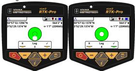
5. The screen will now revert to the locate screen now you can continue to locate the utility. Continue to collect data as needed. If at any point the feature needs to be changed press the "f" pushbutton to open the data dictionary.
