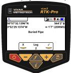
6. Press the "+" pushbutton to log now the receiver will display the spirit level in order to tilt the receiver to align the GNSS antenna.
