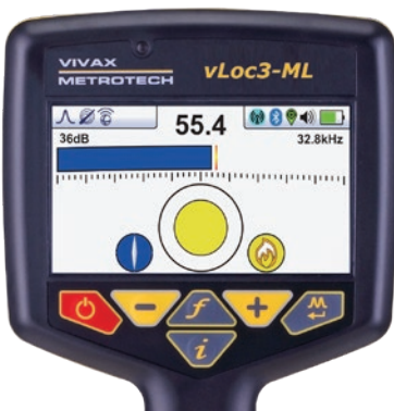
Dual marker and line locating mode screen with circular indicator for marker signal strength and marker type symbol as well as compass and bar graph indicator for line locating
